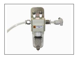
Fill lubrication reservoir with the supplied lubrication fluid. Make sure not to over fill the reservoir or spillage will occur. After filling, be sure to tighten the oil reservoir cap.
