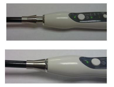
Step 2: Place the light shield over the light guide. Secure the shield over the light guide chuck.
